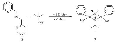
Fig. 4. Synthesis of bis(methylzinc)t-butylamide-bis(2-pyridylmethyl)amide 1.
