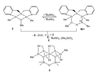
**Fig. 10.** Reaction of **1** with *t*-butylamine in the presence of adventitious silicone grease.
