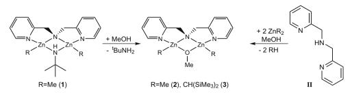
Fig. 6. Synthesis of bis(alkylzinc)methoxide-bis(2-pyridylmethyl)amides (2/3).
