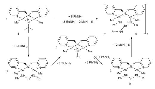
Fig. 8. Aminolysis of 1 with aniline and subsequent degradation to 4.
